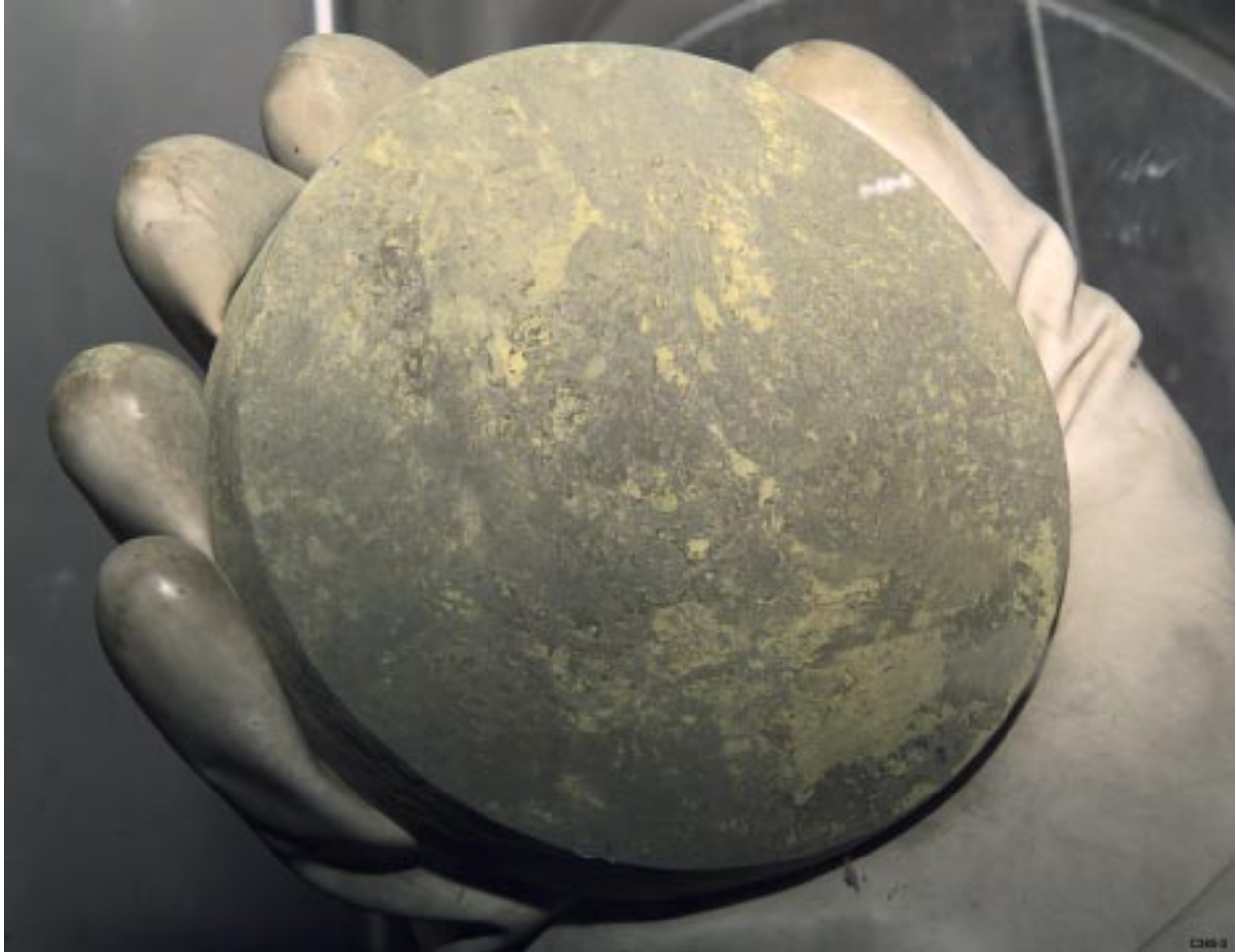
Figure 19 – Pu ingot after six thermal cycles showing moderate surface oxidation.
