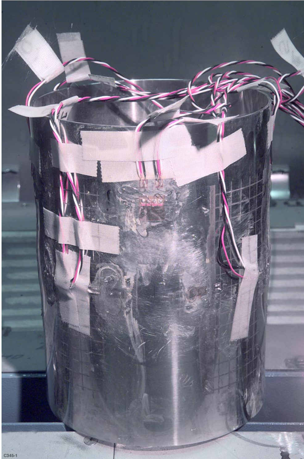
Figure 18 – Cylinder after six thermal cycles. Note plastic deformation around center of cylinder. Cylinder is 6" in length.
